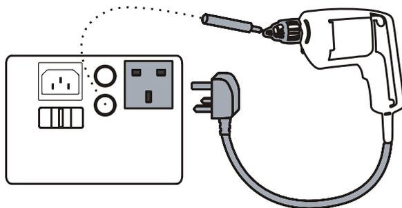
Figure 6. Substitute Leakage Current Connections
